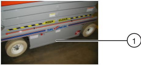
Figure 2-7. Pothole Protection Device
